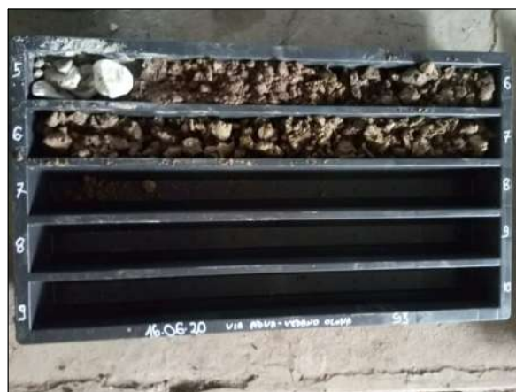
Sondaggio S3 da 5,0 m a 7,0 m da p.c.
