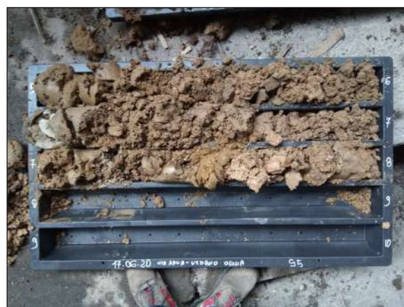
Sondaggio S5 da 5,0 m a 8,0 m da p.c.
